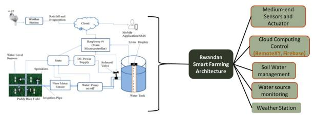
Figure 2: Smart Irrigation architecture deployed for a rice farm in Rwanda. Source (Bamurigire et al., n.d.)
